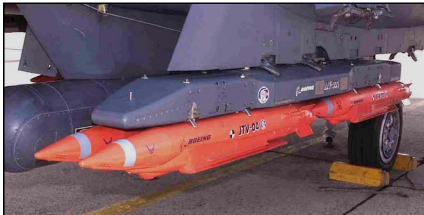
Photograph: F-15E with Boeing SDB's mounted on a Sargent Fletcher Pneumatic Weapons Carriage
