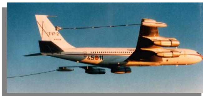
Spanish B-707T/T Trailing Hoses from Wing Pods
